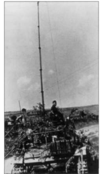
Panzerbefehlswagen Ausf F or H with both the original tubular aerial plus the newer telescoping type with guy-wires. Neither aerial was very practical but sufficed to give the Germans superior tactical command and control. (History in the Making)
